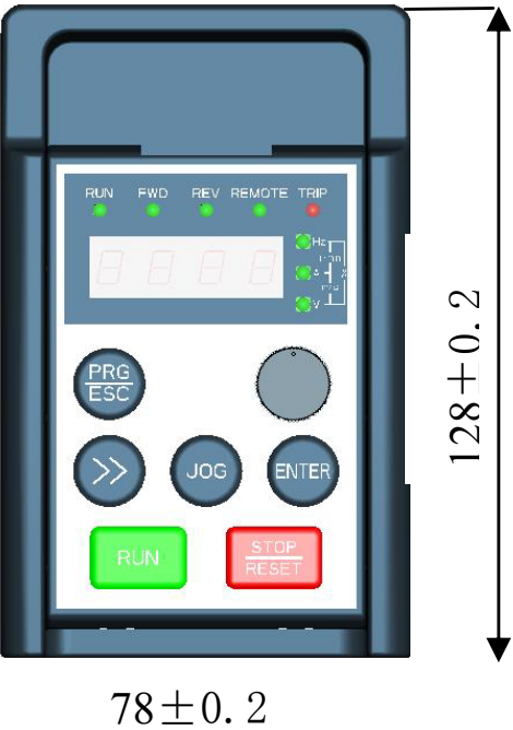
Figure A4-2 Keypad’s tray Installation Dimension (Unit: mm)
