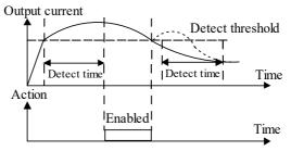
Fig. 5-13-2 Overload pre-alarm function
