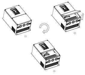
Fig. 2-8 Disassembly schematic diagram of 30kW and above
