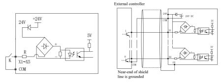
Fig. 2-21 Wiring diagram of multi-function input terminals
