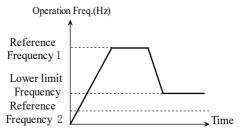
Fig. 5-2-3 Running at lower limit frequency
