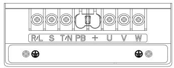
Fig. 2-10 Wiring of terminals of main circuit of 1PH 220V 1.5&2.2kW 3PH 380V 0.75-2.2kW
