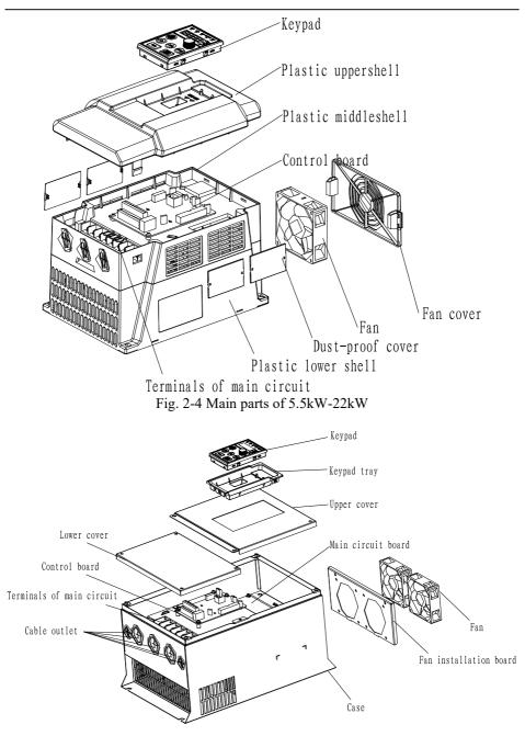
Fig. 2-5 Main parts of 30kW and above
