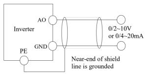
Fig. 2-18 Wiring diagram of analog output terminals
