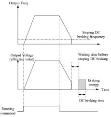
Fig. 5-1-7 DC braking
