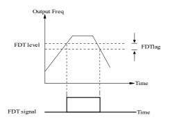
Fig. 5-3-9 Frequency detection FDT
