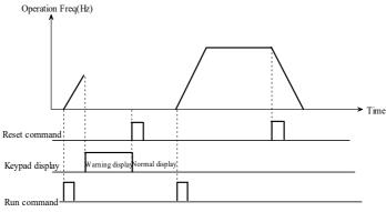
Fig. 5-3-1 Terminal reset
