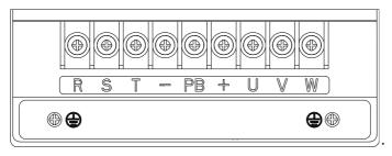
Fig. 2-11 Wiring of terminals of main circuit of 3PH 380V 4-kW
