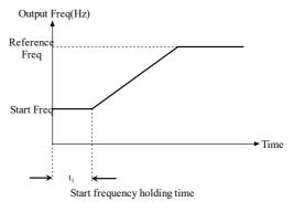
Fig. 5-1-3 Starting frequency and starting time
