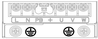
Fig. 2-9 Wiring of terminals of main circuit of 1PH 220V 0.4&0.75kW
