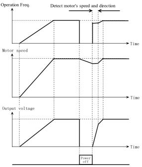
Fig. 5-1-2 Rotating speed tracking restart
