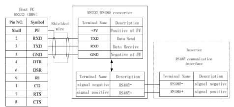
Fig. 2-19 Illustration of wiring between the upper computer and the inverter interface
