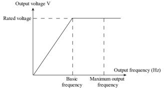
Fig. 5-0-1 Relationship between output frequency and output voltage
