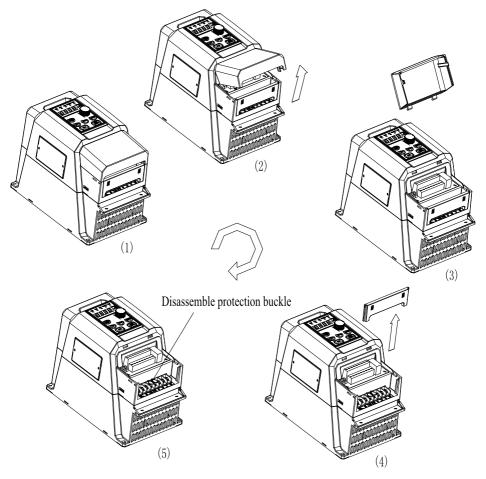
2.3.2 Schematic diagram of connection and disassembly main circuit terminals
