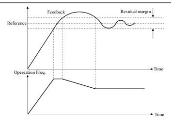
Fig. 5-7-1 Residual margin diagram
