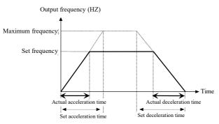
Fig. 5-1-5 Linear acceleration/deceleration
