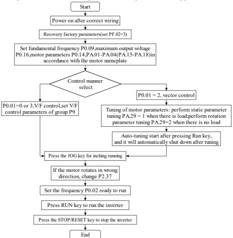
Fig. 3-7 Operation process of inverter first test run operation
