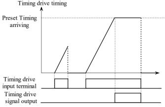
Fig. 5-3-7 Timing driving input
