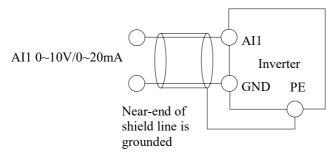
Fig. 2-17 Wiring diagram of analog input terminals
