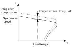
Fig. 5-9-4 Auto slip compensation diagram
