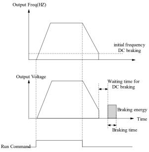
Fig. 5-3-5 DC braking
