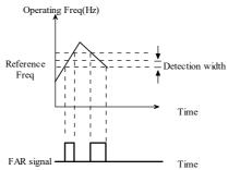
Fig. 5-3-8 FAR detection diagram
