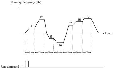
Fig. 5-5-1 Stop mode after single cycle of PLC
