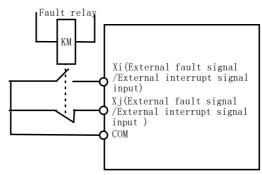
Fig. 5-3-6 Normally open / normally closed
