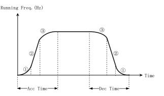
Fig. 5-1-6 S-curve acceleration/deceleration
