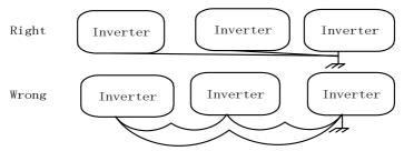
Fig. 2-13 Earthing Connection Method
