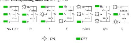
Fig. 3-2 Combinations of unit indicator and their means
