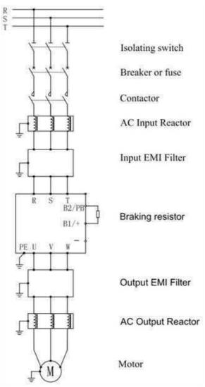
Fig. 7-1 S2R4GB~3022GB/3022PB Peripheral Equipment Connection Diagram
