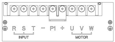
Fig. 2-12 Wiring of terminals of main circuit of 3PH 380V 37-160kW
