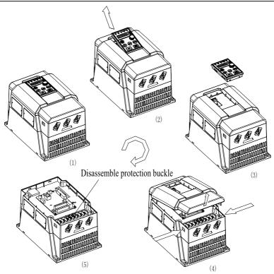
Fig. 2-7 Disassembly schematic diagram of 5.5kW-22kW
