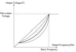
Fig. 5-9-1 Torque-reducing curve
