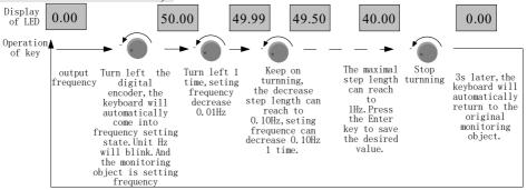
Fig. 3-4 Flow chart of frequency setting
