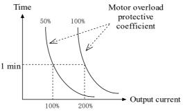
Fig. 5-13-1 Motor overload protection curve
