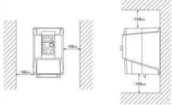
Fig. 2-2 Installation Direction and Space
