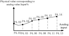
Fig. 5-4-2 Analog input non-linear curve
