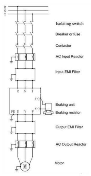
Fig. 7-2 3030G/3030P and above Peripheral Equipment Connection Diagram
