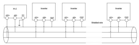
Fig. 2-20 Recommended wiring diagrams (inverters and motors are all well grounded) when PLC is in communication with multiple inverters
